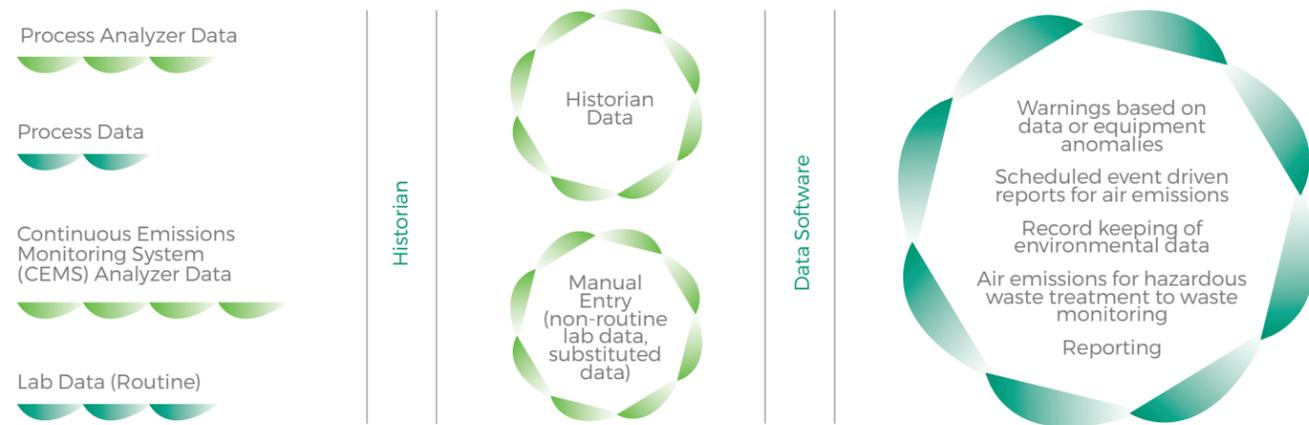
The system ensures that accurate data is produced and makes all required air emission information readily available for all internal and external stakeholders. The system is designed to provide a continuous real-time flow of information and alerts of potential issues, in addition to the standard periodic reports.
